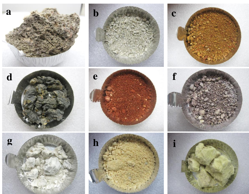
Figure 12: Dried samples in aluminum trays. These represent the sample types listed in Table 2. (a) Altered basalt, (b) white precipitate, (c) orange precipitate/sediment, (d) gray mud, (e) red sediment, (f) purple sediment, (g) clay-rich, (h) silica-rich, and (i) sulfur-rich.
